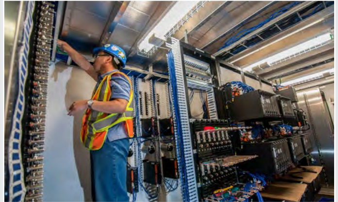
PNR RailWorks Signals & Communications Division constructed, wired and tested all 37 bungalows for the Georgetown South project in its Guelph, ON, wiring shop.
